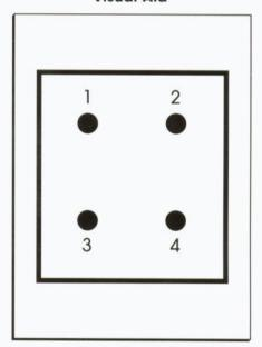
U-Bolts must be tightened and torqued using a cross pattern sequence.
